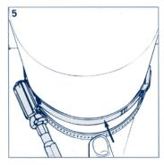
Hold down any excess band just before the buckle is clamped. Finally tighten with the ratchet spanner.
