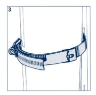
Engage the band into the screw housing and screw band through by approximately 50mm.
