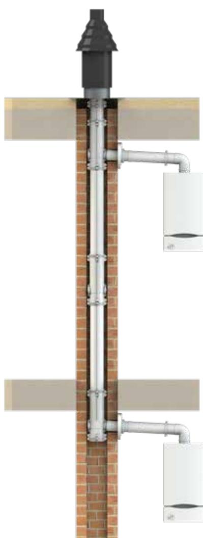
**2 SET AND INSTALL** By using the pre-marked scales on the flue gas pipe, the floor to floor heights can be set.
